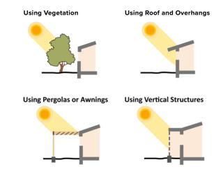
Figure 3-5. Examples of façade screening and external shading. Source: © AtkinsRéalis, 2025
