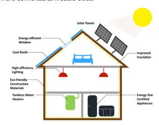
Figure 3-4. Features of an energy-efficient home. Source: © AtkinsRéalis, 2025
